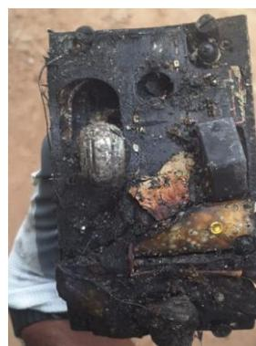
Figure 12 Landing Gear Lever Module
