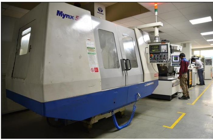
Exhibit 39: CNC machine used to mold H13 steel, basis design team working;
